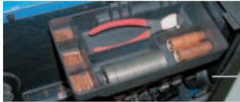
**Removable consumable compartment and access to wire drive system** located under side door.
