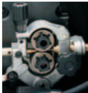
**Industrial, dual-gear-driven, cast-aluminum drive system** features no-tool, quick-change drive rolls and an easy-to-set tension adjustment knob with a scale for consistent settings.
